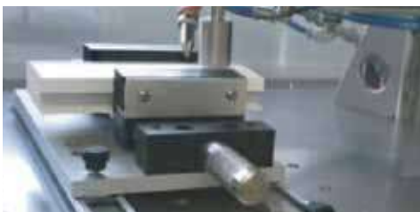
Easy sample clamp with a X-table
